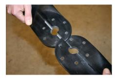
Propeller halves slide together
