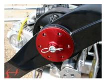
Quick release propeller mounting
